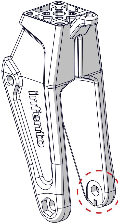
This is the 7" Wheelhouse. Before being able to use this part, you need two Nock Washers M8-16. Press these washers into the slots.
