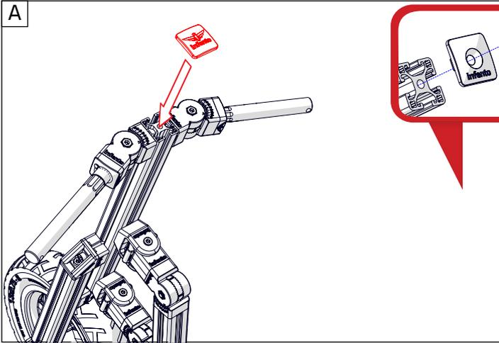
If your protect cap has a hole, use a M8x12 countersunk bolt to fasten it
