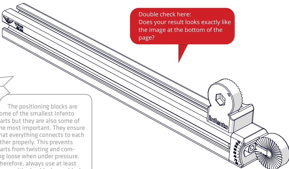
The positioning blocks are some of the smallest Infento parts but they are also some of the most important. They ensure that everything connects to each other properly. This prevents parts from twisting and coming loose when under pressure. Therefore, always use at least two positioning blocks per block.
