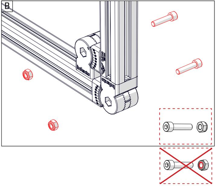
There are two different knurled discs. One for each corner ending in a 5 (5-15-25-etc. degrees), which has one stripe round the outside, and one for each corner that ends in a 0 (0-10-20-etc degrees), which has two stripes round the outside.
