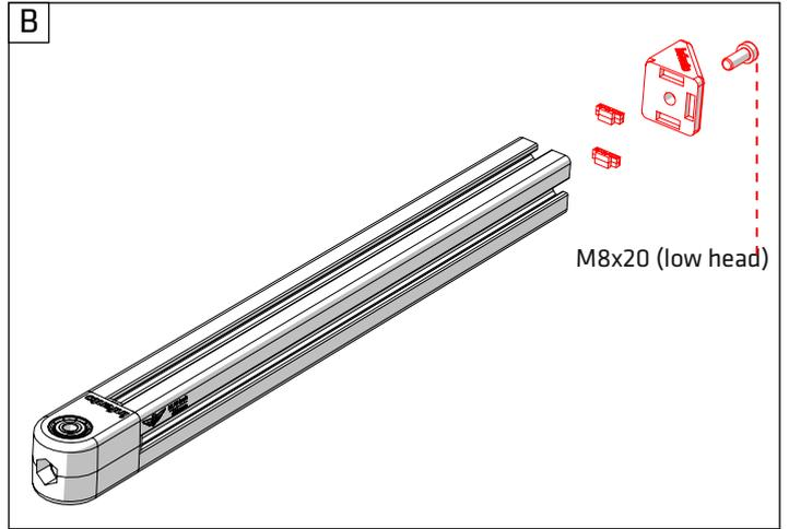
Use the Allen key handle so you can tighten the bolt well.
