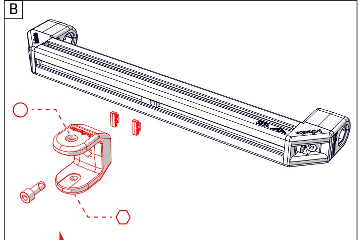
When tightening the bolt always check whether the profile nut remains perfectly straight in the slot. If this becomes crooked, you can push against the side of the profile bolt with the Allen key to correct this.
