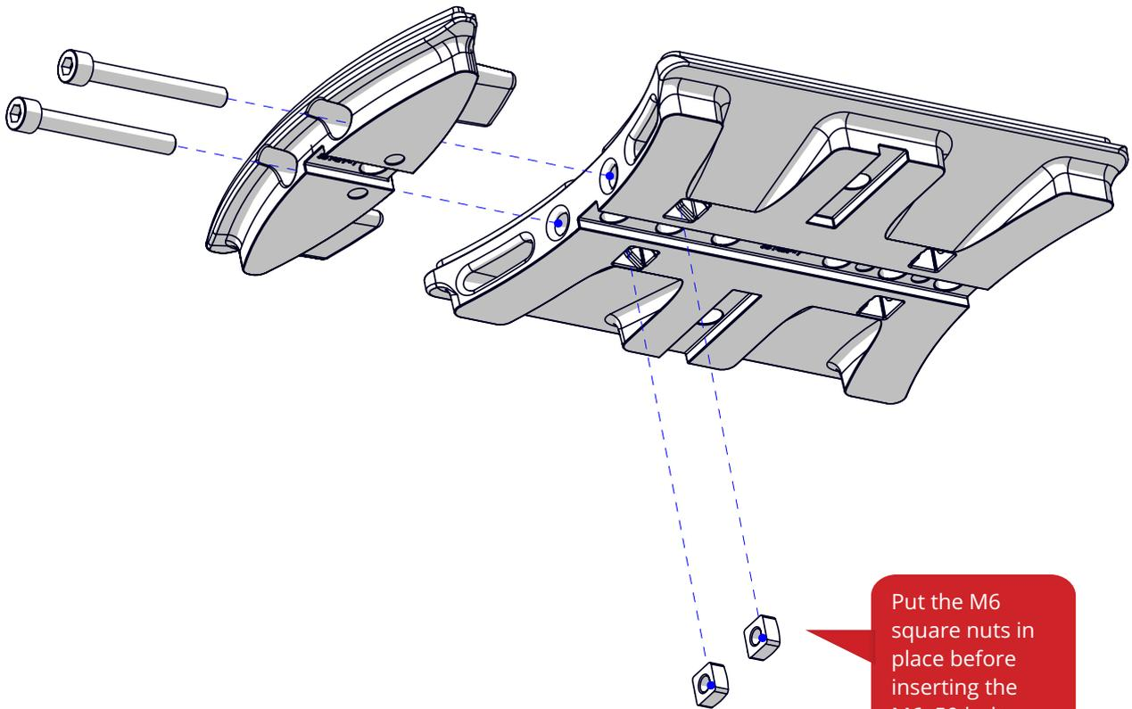
Put the M6 square nuts in place before inserting the M6x50 bolts.
