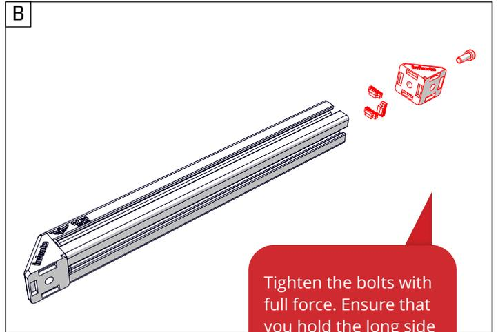
Tighten the bolts with full force. Ensure that you hold the long side of the Allen key in your hand as this enables you to exert greater force.
